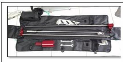
Gambar 1. Alat *Dynamic Cone Penetrometer* (DCP)
